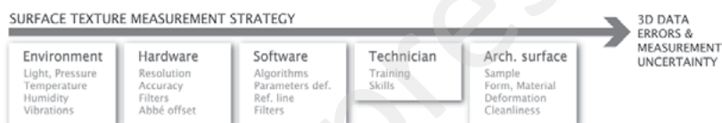
FIGURE 2: EXAMPLE OF SOURCES OF MEASUREMENT ERROR IN SURFACE TEXTURE THAT LEAD TO UNCERTAINTY OF MEASUREMENT RESULTS.
