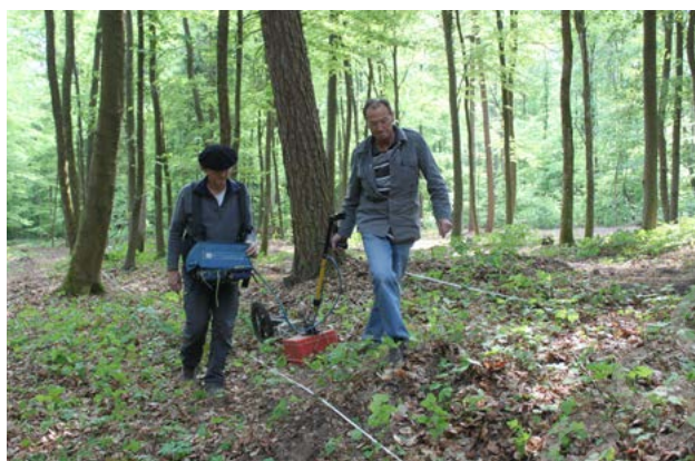
FIGURE 3: GROUND PENETRATING RADAR WITH 400 MHZ ANTENNA IN RUPPERTSHÜTTEN, 'KLOSTER EINSIEDEL', GERMANY. (HARALD ROSMANITZ, SPESSART ARCHAEOLOGICAL PROJECT).
