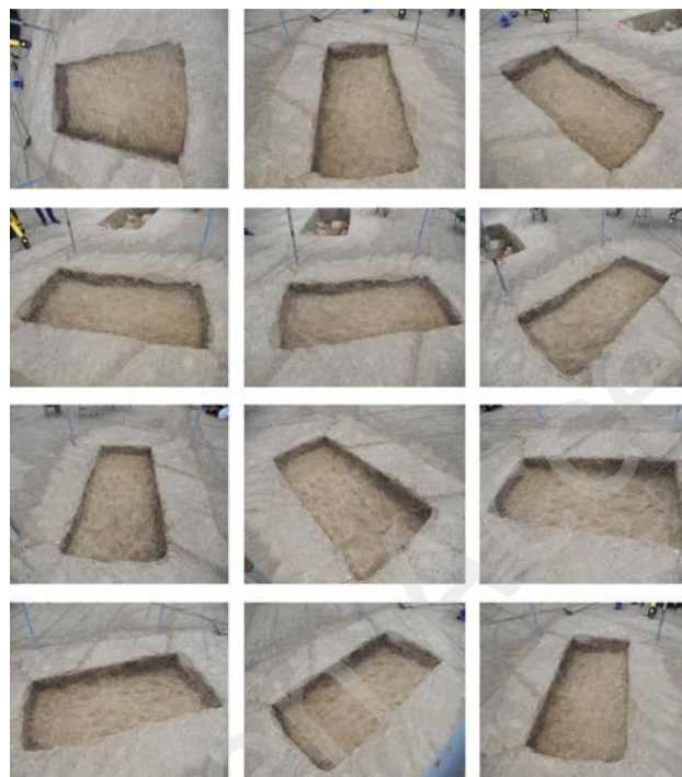
FIGURE 5: EXAMPLE OF A PHOTO SET. THE SURVEYING PROJECT ENVISAGED TAKING 12 PHOTO SETS FOR EACH EXCAVATION STAGE. THE NECESSITY OF OVERLAPPING TWO OR THREE PHOTOGRAMS WAS TAKEN INTO ACCOUNT.
