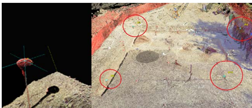
FIGURE 9: GEOREFERENCING THE TLS RANGE DATA BY GCPs AND EXCAVATION GRID.
